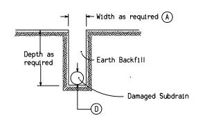
(A)= A minimum of 24" shall be excavated outside the normal utility trench wall or such greater width as may be required to expose a minimum of 12" of undamaged drain tile.
