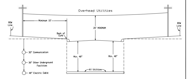
Notes: Utilities shall be located between back of curb and the highway row. Utilities should be located as near to the highway row line as practical. See Utility Policy, Section 115.13 for further details.
